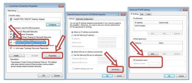
If it is not possible to change the metric, you have to change your IP settings. The factory default AS55X IP address is 192.168.0.2. If the AS55X is configured to another IP address, you have to use USB local access or reset the AS55X by using the reset button.
