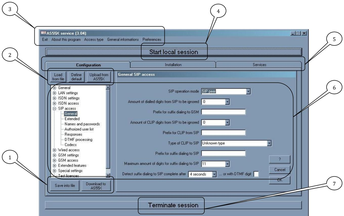
1. Buttons to save current configuration or to download configuration to AS55X
