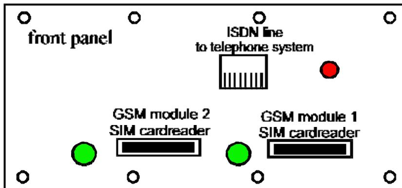
RJ 45 jack for connecting the ISDN line of the PABX, internal or external ISDN line, point to point or point to multipoint connection
