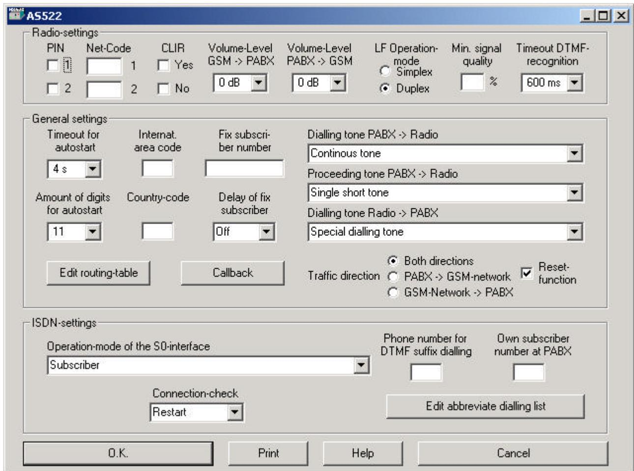
On the 3,5'' disk you find the configuration software. You need to install it through setup.exe. Connect a COM port of the PC to the RS232 interface of the AS 52X by using a standard serial cable cord (9 pin plug ↔ 9 pin jack connected pin1↔1, pin2↔2, pin3↔3 and so on). Connect the AS 52X to the power supply. The AS 52X starts with auto-power on. If not, check the power supply (esp. bridge between pin 7 and 8 of the connector).
